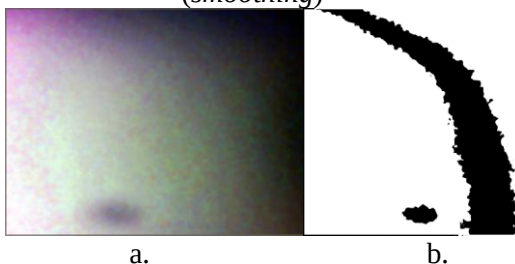
Gambar 12. Pengolahan citra thresholding (a) smoothing & (b) thresholding .
