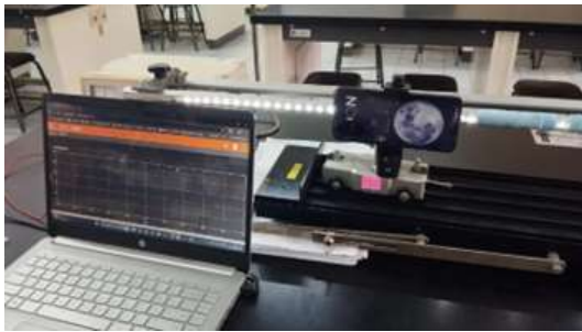
Figure 3. Experimental setup for uniformly accelerated motion using phyphox
