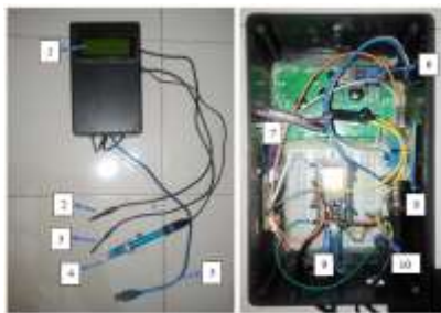
Gambar 3. Realisasi Alat Sistem Monitoring Kualitas Air Tambak Udang, (1) LCD 20x4, (2) probe sensor TDS, (3) probe sensor DS18B20, (4) probe sensor pH, (5) Kabel Micro USB, (6) Modul LCD I2C, (7) Modul sensor TDS, (8) Modul Sensor pH, (10) Resistor 4,7 k \Omega
