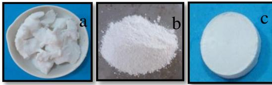
**Gambar 4.** Komposit MgO-SiO<sub>2</sub> (a) gel MgO-SiO<sub>2</sub>, (b) powder MgO-SiO<sub>2</sub>, (c) pellet MgO-SiO<sub>2</sub> telah disinterring.
